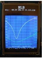
The plot shows the return loss of the DUT over the frequency scan range as a white trace plotted against the scale on the left of the plot area. The green trace is the computed VSWR plotted against the scale on the right of the plot area. The lowest calculated VSWR and the associated frequency are rendered in green at the bottom of the plot area (1.02 @ 14,233,959 in this case).
