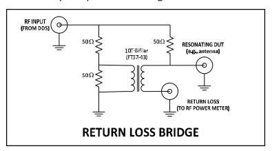
I built my RLB on a small one-sided, perforated board using, what I call, a "Carved Circuit Board" ("CCB" as opposed to "PCB").
