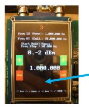
8. Tapping anywhere on the Freq Hi line will change the frequency to 31 MHz (note the change in signal amplitude).
