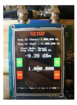
7. Pressing End on the keyboard will change the frequency to 31 MHz (note the change in signal amplitude).
