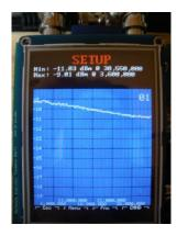
12. Press Escape twice to go to Terminal mode and press Ctrl-C to capture the calibration data in the calibration data buffer and save it to EEPROM. The calibrated calibration curve will then be plotted with the calibration applied (A straight line at 0.00 dBm).
