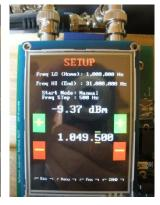
Press Escape to exit sig gen mode, Scroll Lock to enter Command mode, and F1 to bring up the SETUP PLX form. Press Page Down to go to page two. Delete the Signal generator op mode. Press Enter to save the change.
