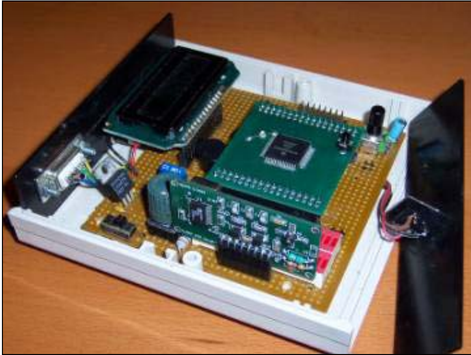
This photo shows the DDS Daughtercard included in the Exerciser ... which is a test fixture that all HC908 Daughtercards get plugged into in order to get tested and qualified before being programmed with the appropriate software before shipping.
