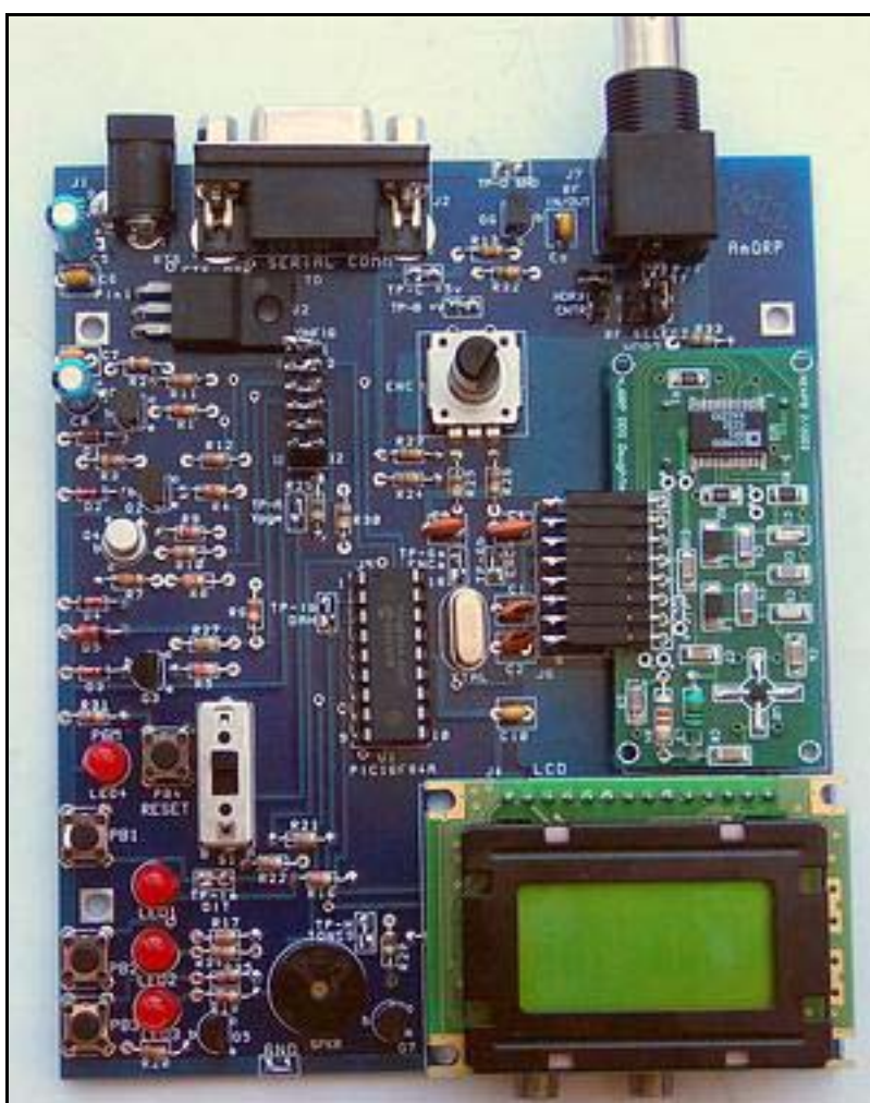
DDS card plugged into the PIC-EL project board. (The DDS card shown here is the original "DDS-30" Daughtercard ... the new DDS-60 card is plug-compatible on the PIC-EL hardware.)
